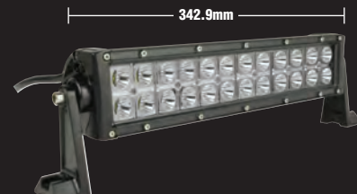
RTXBC272 13.5" • 6480 lumens • 3A 72W (24 DEL/LED x 3W)
