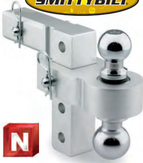
ALUMINIUM / ALUMINUM 6,000 lb SB2925 Boules / Balls : 1 7/8" & 2" SB2926 Boules / Balls : 2" & 2 5/16" Trou de boule / Ball hole 1" Baisse / Drop 6" Hausse / Rise 6"
